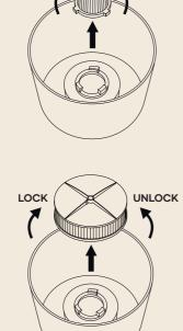
Clean the filter by turning it anti-clockwise to unlock and remove, then tap gently to release fine dust.
