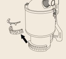
Regularly remove and clean the external motor filter.
