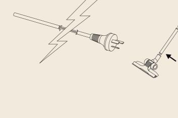
Check all power cords and ensure there are no cuts, abrasions or exposed wiring. \*Refer to cord management below.
